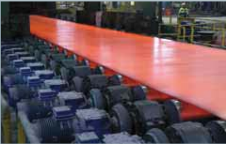
5 Rougher exit roller table
