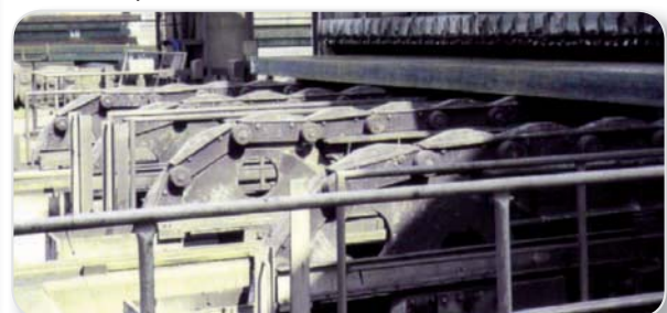
Special chain pitch 600 mm pre-heating frames. ( Oven temp. 500° C)
