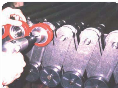
Passenger Escalator chains pitch 203.20mm 506 kN tensile strength.
