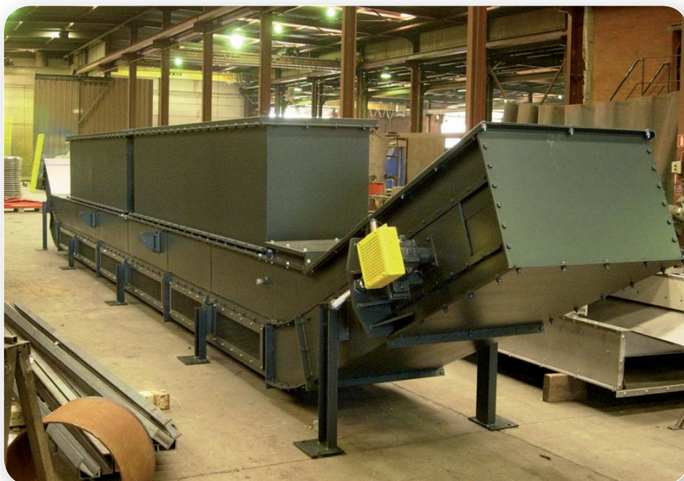
Scrapper conveyor casing for extraction under bunker or hopper.
